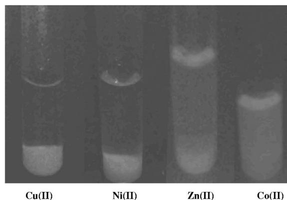
Fig. 1. Equilibrium batch protein uptake. Each tube contained 1 ml cell extract containing GFPuv, 3 ml phosphate buffer (top phase), pH 7.5, 2 ml IMAC resin (bottom phase) charged with, from left to right, Cu(II), Ni(II), Zn(II) and Co(II). Absence of fluorescence in upper phase indicated GFPuv adsorption.
