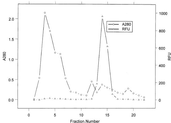
Fig. 6. Ni(II)-IMAC with 1.0 M NaCl in mobile phase. Fractions 1–10 phosphate buffer, pH 7.5. Fractions 11–20 pH elution (7.5 to 6.0).
