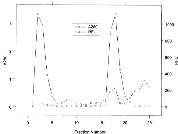
Fig. 7. Ni(II)-IMAC with 2.0 M NaCl in mobile phase. Fractions 1–10 phosphate buffer, pH 7.5. Fractions 11–20 pH elution (7.5 to 6.0). Fractions 21–25 phosphate buffer, pH 6.0.
