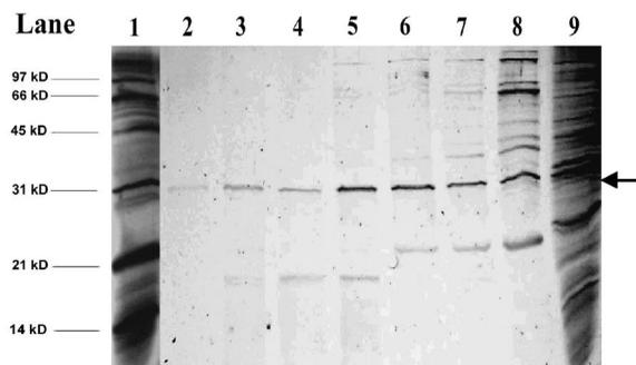
Fig. 5. SDS-PAGE of Ni(II)-IMAC with 0.25 M NaCl in mobile phase. Lanes 1 and 9 contain molecular mass standard and cell extract containing GFPuv (arrow indicates GFPuv mobility). Lanes 2–8 contain pooled Ni(II)-IMAC fractions from pH gradient. Lanes 5 and 6 correspond to the major peak of GFPuv at pH 6.5. kD=Kilodalton.
