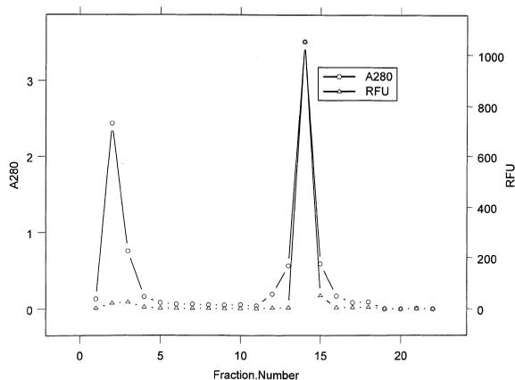
Fig. 2. Cu(II)-IMAC with 0.25 M NaCl in mobile phase. Fractions 1–10 phosphate buffer, pH 7.5. Fractions 11–20 imidazole gradient (5 to 70 mM).
